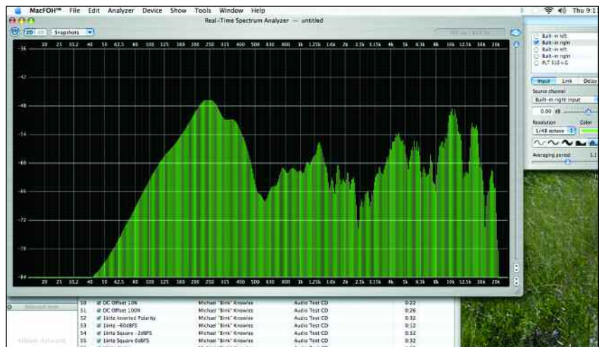
Figure 2: Measured 1 meter 1/48 octave response of the same loudspeaker system. Comb filtering peaks and valleys of as much as 24 dB are now apparent in the higher frequencies due to the overlap in pattern between the two closely situated full range loudspeakers, as well as room modes and placement of the measurement microphone. While the low frequency buildup centered on 250 Hz can probably be solved with equalization, it is now apparent that the problems in the higher frequencies are due to improper loudspeaker placement and attempting to equalize them would only change the loudspeakers' tonality for the worse.
